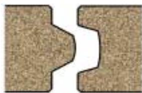
groove and tongue joint profile
