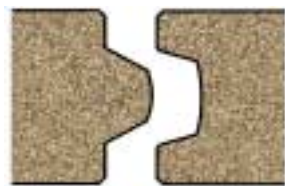
groove and tongue joint profile
