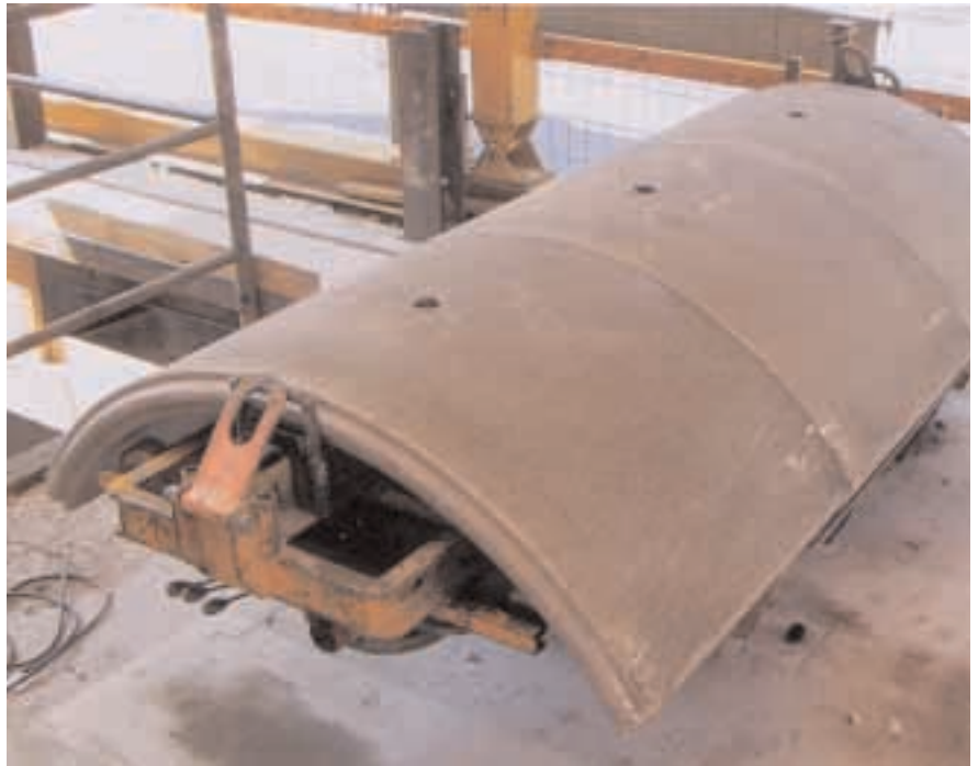
3 Pre-fabricated tubbings for the DN 1300 sewer (photo: Meyer Rohr+Schacht)
